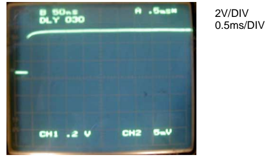
Measuring point: TP6 on TRS.A board Frequency: 75 kHz
